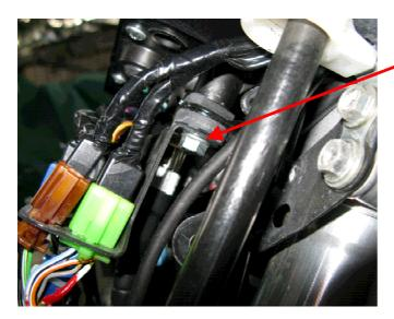
After removing the front visor with the headlight, remove the 2 nuts locating the speedo & wiring harness brackets. This view shows only the left side nut.
